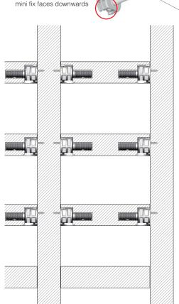
Also suitable for top and bottom panels when a back panel is used.
