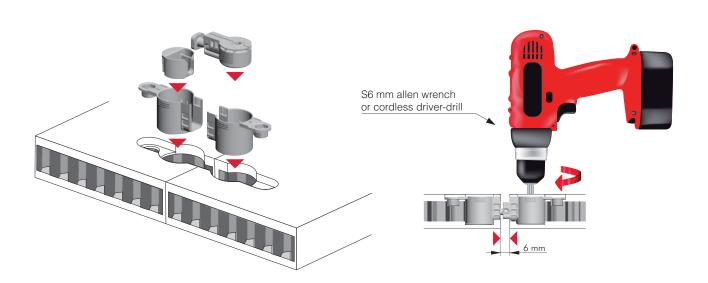
Captivating painted cover cap to be placed in position for connecting free standing shelvings together.
