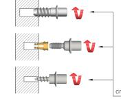
Assembling with threaded pin to achieve horizontal connection
