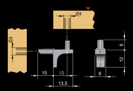
With Ø4mm pin and Ø4mm shelf-fixing lug.
