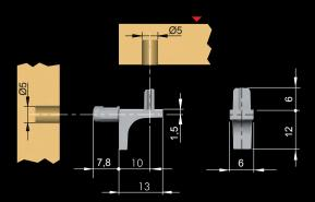
With Ø5mm pin and Ø5mm shelf-fixing lug.
