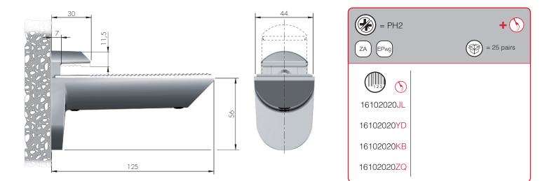
NOTE: KAIMAN is supplied in carton box including 2 pieces, accessories and fitting guide. Countersunk fixing screws  $\emptyset$  5x50 and rawlplugs Fischer SX  $\emptyset$  8x40 to wall are included.
