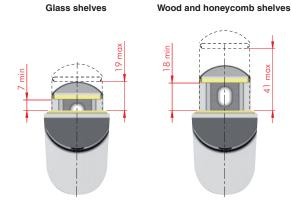
Shelf is clamped between a layer of ridged plastic on both the lower and upper side (coloured parts).
