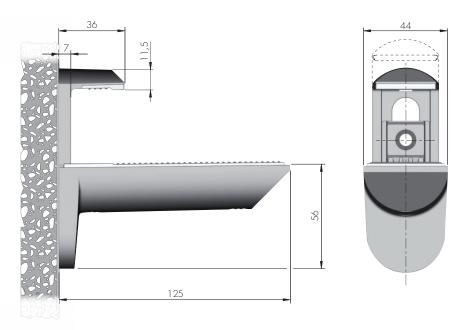
NOTE: KAIMAN MAXI is supplied in carton box including 2 pieces, accessories and fitting guide. Countersunk fixing screws Ø 5x50 and rawlplugs Fischer SX Ø 8x40 to wall are included.
