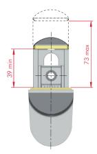
Shelf is clamped between a layer of ridged plastic on both the lower and upper side (coloured parts).
