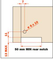
REAR NOTCH with Push Synchronizer and tilt adjustment lever
