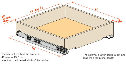
For drawer sides with sub-fronts between 12 and 13 mm, we recommend the use of the build-up spacer **AFSFXXB**.
