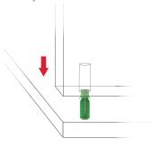
5 - The two panels will be permanently assembled without using any kind of glue.
