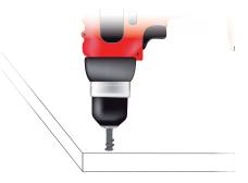
2 - Make Ø 5mm face borings on the other panel.  $\boldsymbol{3}$  - Screw the assembly fitting into the face bored panel
