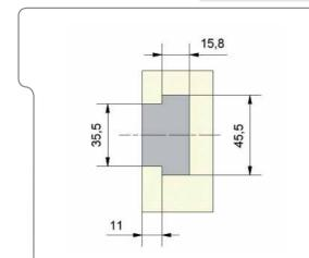
A B Slide completely recessed B+23 mm Door thickness +0.5 mm
