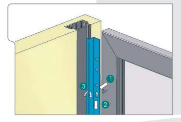
Insert the two Slides into the grooves in the side panels of the cupboard. Once the cupboard structure is assembled attach the door to the bracket by screwing the screws into the slots 1 and fitting the door 2 onto them. Check that the doors are parallel and, once in the correct position, tighten the screws 3. For greater stability of the door additional holes may be made in the bracket.
